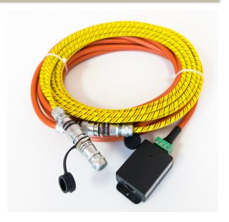
The Conteg Rope Water location sensor is designed for specific location water detection. It can be connected to Ramos Optima or Ramos Ultra's RJ-45 Intelligent Sensor ports, enabling the unit to detect the specific location of water ingress.
